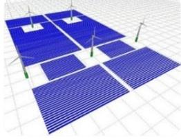
**Wind-PV-hybrid systems** combine the use of wind energy and photovoltaic (PV) within a power plant. **Surface-and grid infrastructure are jointly used in an efficient way.** In addition, the PV and wind power profiles complement each other over the course of the year, resulting in **more stable power generation.** Such hybrid power plants on a gigawatt scale are currently being built in multiple regions around the world, particularly due to the low production costs of both technologies.
